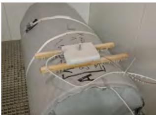
LIFERAFT STORED FOR 50HRS AT  $-70^{\circ}\text{C}$
